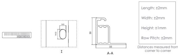
For detailed sizes and tolerance specification, please consult detailed module drawing
